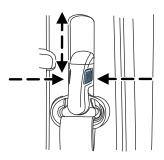
**WARNING:** Position the safety belt height adjusters so that the belt rests across the middle of your shoulder. Failure to adjust the safety belt properly could reduce the effectiveness of the safety belt and increase the risk of injury in a collision.
